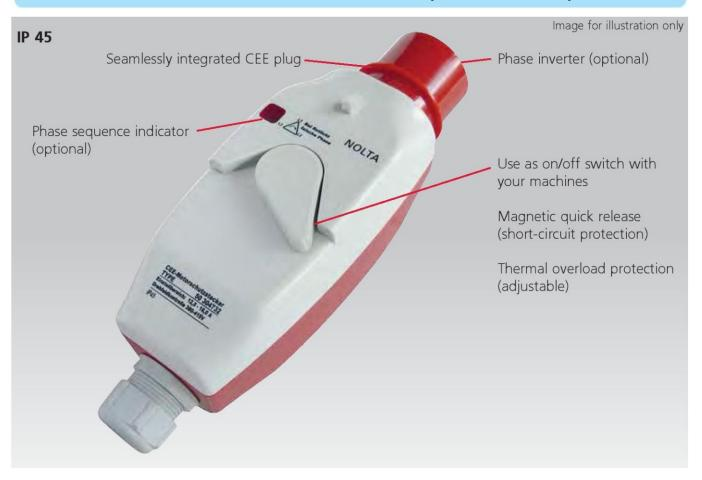
The NOLTA 50 Series Rotary-Toggle is designed for tough building sites and industrial applications, e.g.:
