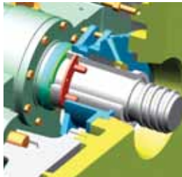
Left: Orange centring tool pins align stuffing box to the sleeve
