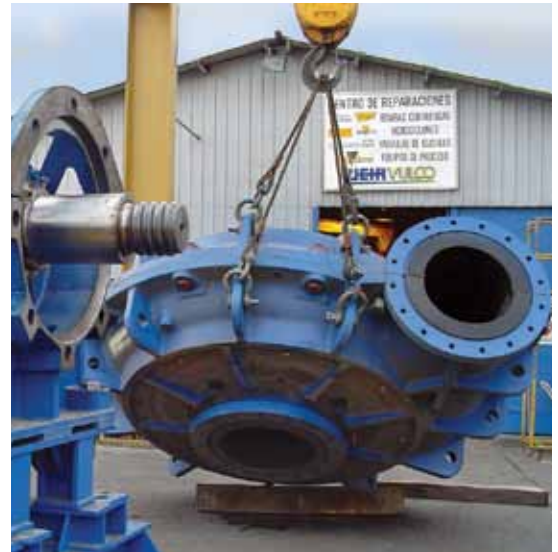
Above: A new innovative quick change procedure has been developed for faster removal of the larger MC range pump wet ends. A 650 MCR wet end being removed in Santiago, Chile
