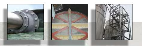
Therefore the Sliding Frame is designed to break any bridges when moving in one direction, and slide under the material when moving the opposite direction, thereby promoting bulk material flow.
