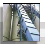
The Saxlund Chain Conveyor is a continuous operating conveyor enclosed within a bolted rectangular cross-section casing. It may be arranged horizontally or inclined with bends to suit the application.
