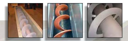
Saxlund Screw Conveyors are an essential part of many conveying and storage systems. Simple design and easy maintenance, screw conveyors successfully move most non-free flowing materials. Saxlund have a long history and experience in the design and construction of Screw Conveyors. We manufacture three main types:
