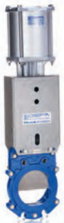
SD 1 DOMINO Schieber/ Knife gate valve AT 100 Beidseitig dichtender Zwischenflansch Plattenschieber aus Grauguss Bidirectional wafer type knife gate valve for installation between flanges, cast iron Baulänge/Face-to-face dimension: EN 558-1, Reihe/Series 20 DN 100 – DN 150, PN 10/16 DN 200 – DN 400, PN 10
