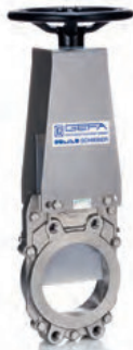
SD 5 DOMINO Schieber/ Knife gate valve AT 150 Anflanschschieber, Edelstahl-ausführung, beidseitig dicht Flanged knife gate valve, stainless steel design, bidirectional Baulänge/Face-to-face dimension: EN 558-1, Reihe/Series 20 DN 50 – DN 150, PN 10/16 DN 200 – DN 400, PN 10
