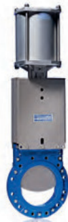
SD 7 DOMINO Schieber/ Knife gate valve AT 200 Anflanschschieber aus Sphäroguss, beidseitig dicht Flanged knife gate valve, ductile iron GGG40, bidirectional Baulänge/Face-to-face dimension: EN 558-1, Reihe/Series 20 und/and 16, DN 50 – DN 1500, PN 10/16
