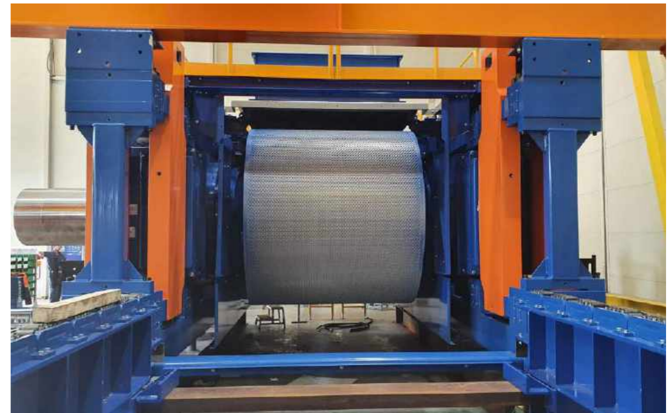
Enduron® HPGR with unique L:D ratio for hard-rock grinding
