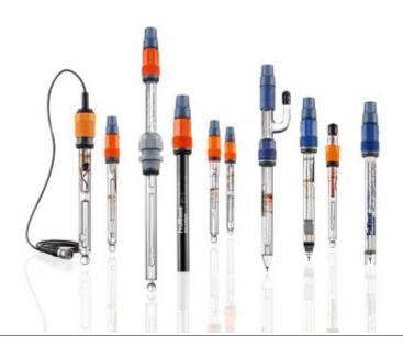
PHEP-H – pH 3...14, max. 100 °C/3 bar, PHEN – pH 1...12, max. 80 °C/pas de surpression, PHES/PHEK – pH 1...12, max. 60 °C/3 bar, PHEP/PHER – pH 1...12, max. 80 °C/6 bar, PHED - pH 1...12, max. 80 °C/8 bar, PHEX – pH 1...12, max. 100 °C/16 bar, PHEF – pH 0...12 max. 50 °C/7 bar
