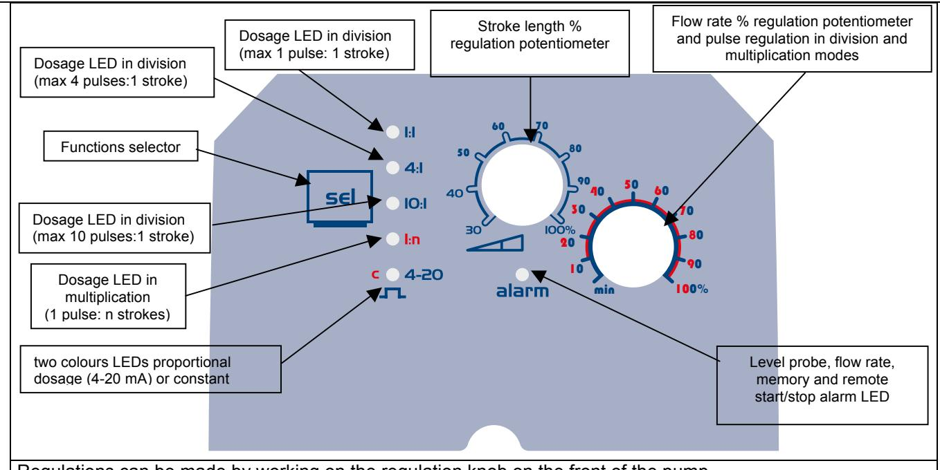
Regulations can be made by working on the regulation knob on the front of the pump
