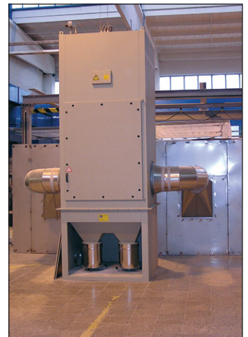
Extraction of a grinding booth by a VARIO 3 eco
