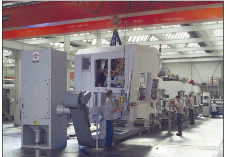
VARO 2 eco for the extraction of chips at an assembly line
