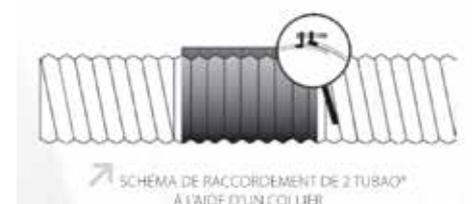
SCHEMA DE RACCORDEMENT DE 2 TUBAO® A L'AIDE D'UN COLLIER
