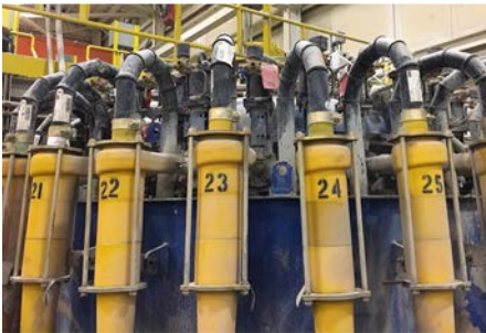
Top: Cavex® 100CVX polyurethane hydrocyclone clusters at an iron ore mine in Brazil.
