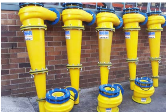
Left: Cavex® polyurethane 250CVX hydrocyclones ready for installation in South Africa.
