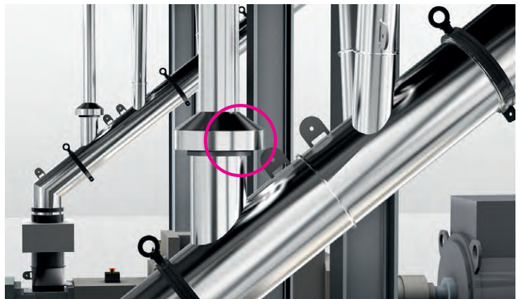
Dust separation with collection hoods at the extruder's feed throats
