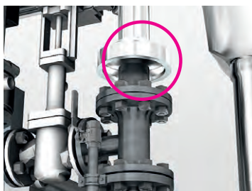
Connection of the fume extraction to the vacuum degassing station
