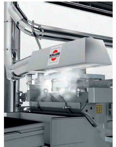
Fume extraction at an extruder
